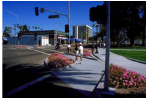
Planters being used to reduce the turning radius and shorten the crossing distance for pedestrians (Oxnard, CA) Dan Burden via the Pedestrian and Bicycle Information Center
