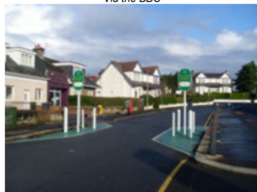
The signs on both sides of the road, as well as the bollards narrowing the road, encourage safer speeds in this residential area (East Renfrewshire, Scotland) Stephen Sweeney via Wikimedia Commons
